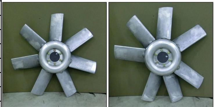
Figure 2: Characteristics of the propellers. Centre: conventional propeller – Right: propeller with irregularly spaced blades
