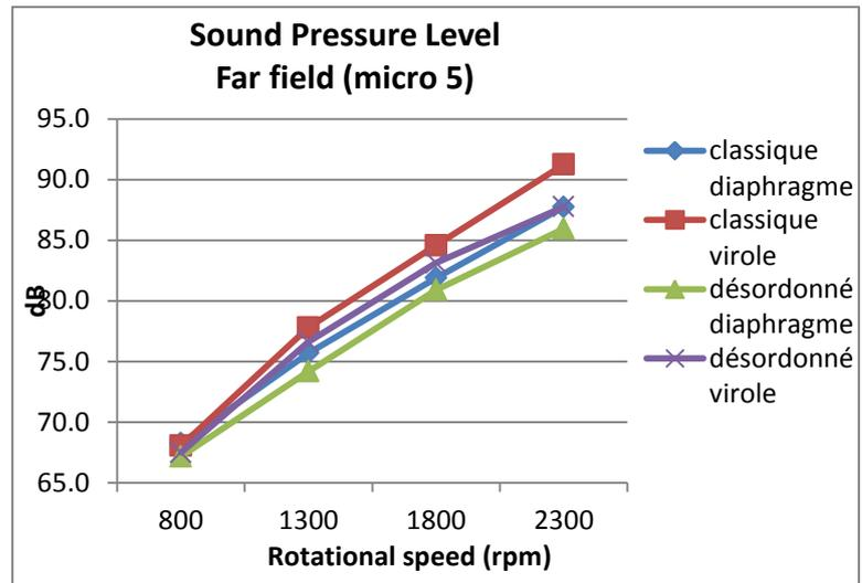
Figure 4: Graph of the sound pressure levels as a function of speed
