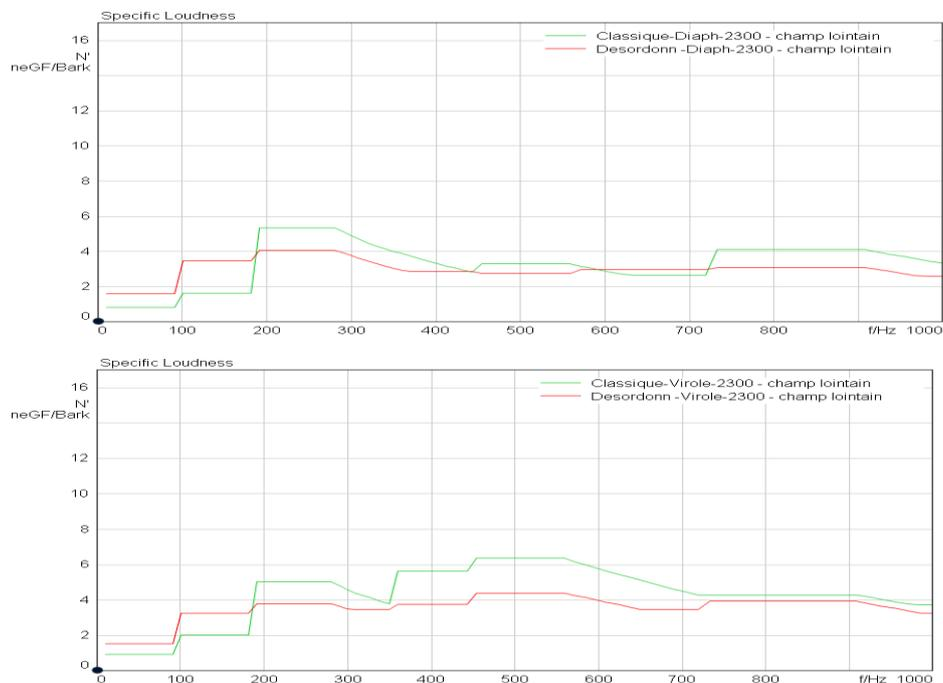
Figure 6 : Loudness - comparison of conventional propeller and propeller with irregularly spaced blades - Diaphragm (top) and Shell (bottom) 2300 rpm
