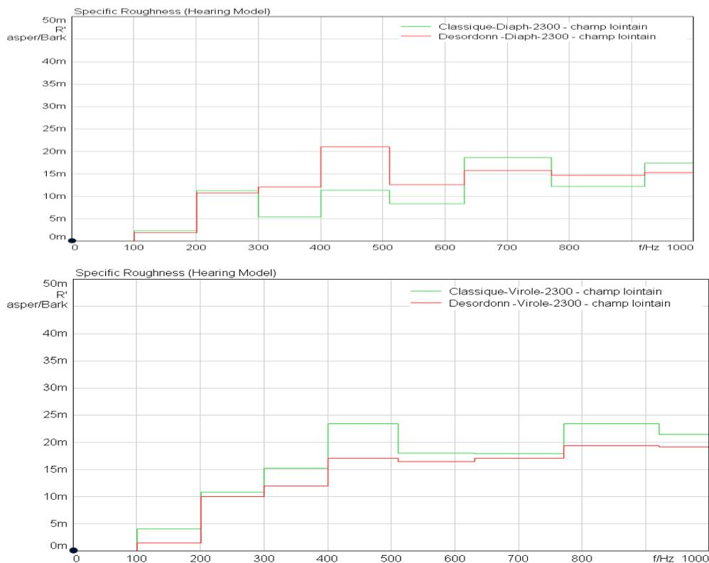
Figure 8 : Roughness - comparison of conventional propeller and propeller with irregularly spaced blades - Diaphragm (top) and Shell (bottom) 2300 rpm
