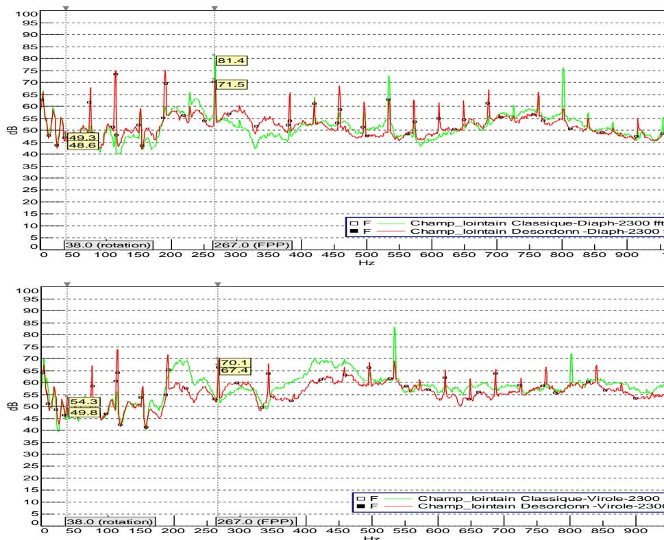
Figure 5: Comparison of conventional propeller and propeller with irregularly spaced blades - Diaphragm (top) and Shell (bottom) 2300 rpm
