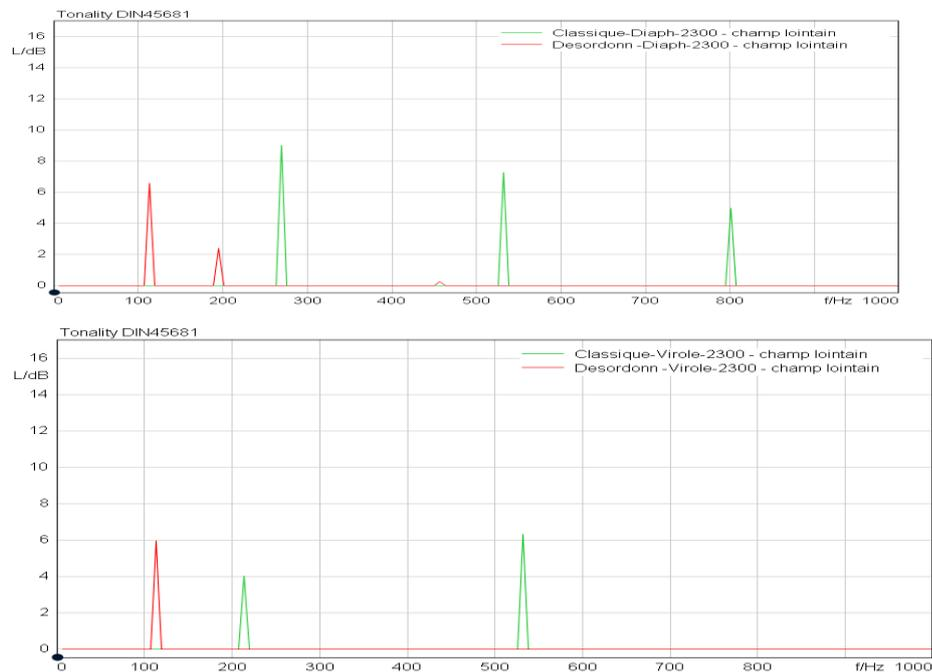
Figure 7 : Tonality - comparison of conventional propeller and propeller with irregularly spaced blades - Diaphragm (top) and Shell (bottom) 2300 rpm
