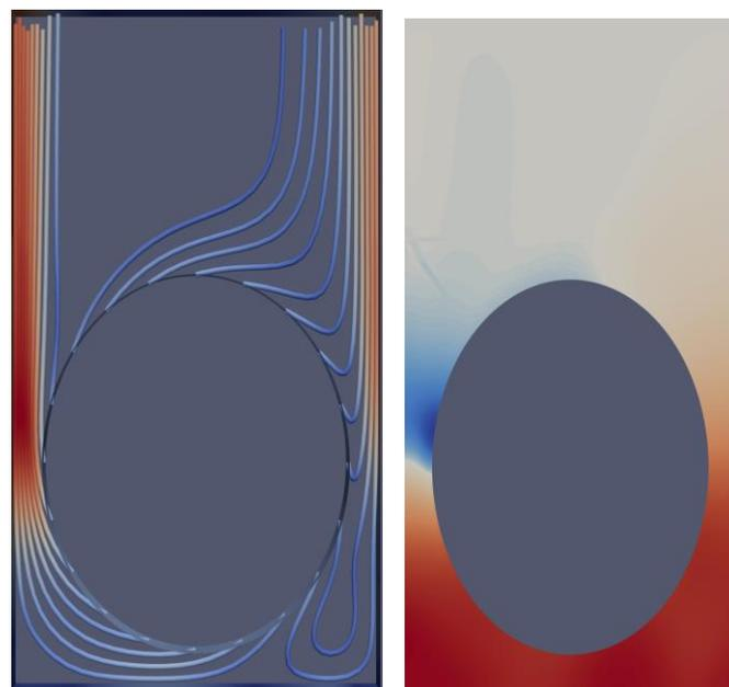
Figure 6: Flow patterns slowrunner  $s/D=0.6$ . Streamlines (left) coloured by velocity magnitude, pressure distribution (right). (Colour map: Maximum values red, minimum values blue)
