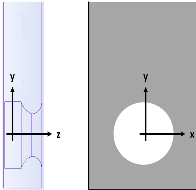
*Figure 1: Plane  $z=0$  used as twodimensional ( $x$ - $y$  plane) computational domain in the simulation*
