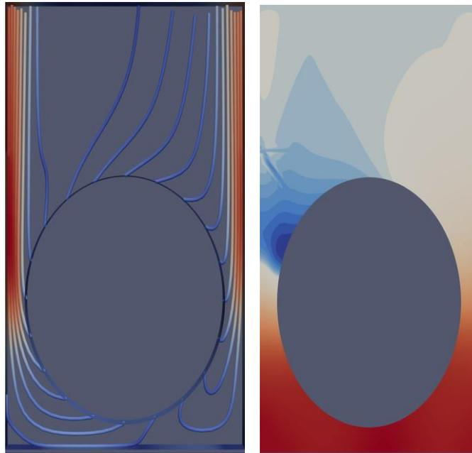
Figure 5: Flow patterns fastrunner  $s/D=0.6$ . Streamlines (left) coloured by velocity magnitude, pressure distribution (right). (Colour map: Maximum values red minimum values blue)
