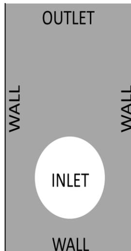
Figure 3: Computational domain with boundary conditions
