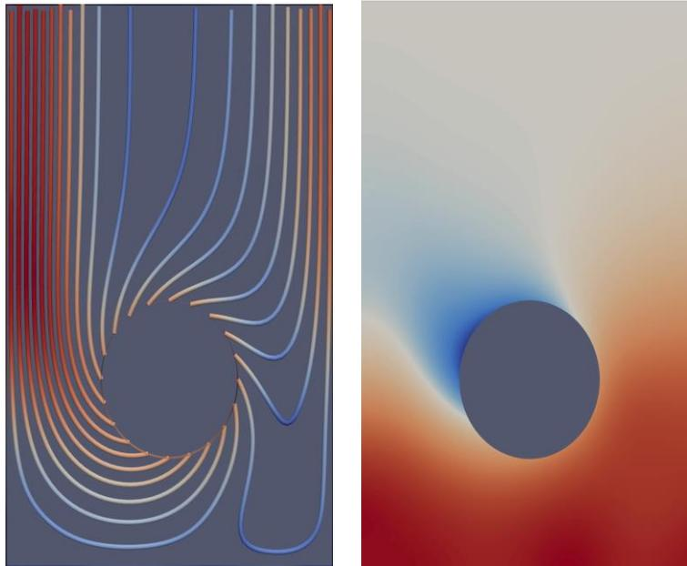
Figure 7: Flow patterns fast runner  $s/D = 1.2$ . Streamlines (left) coloured by velocity magnitude, pressure distribution (right). (Colour map: Maximum values red minimum values blue)
