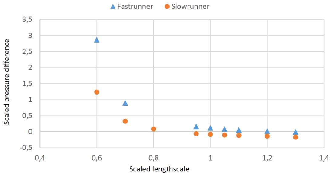
Figure 9: Scaled pressure difference vs. scaled enclosure size for fastrunner and slowrunner
