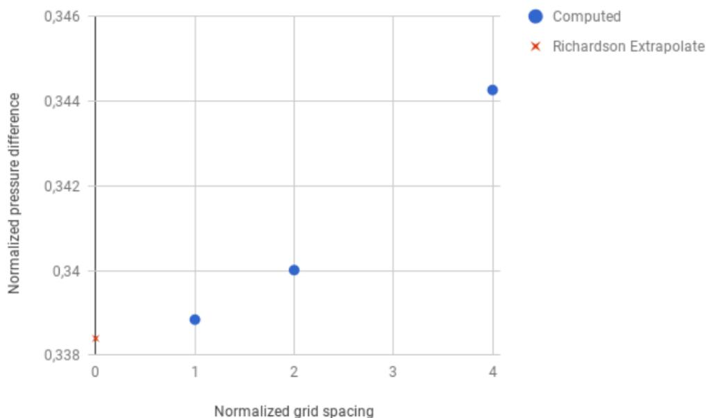
Figure 4: Grid convergence study: scaled pressure difference vs. normalized grid spacing
