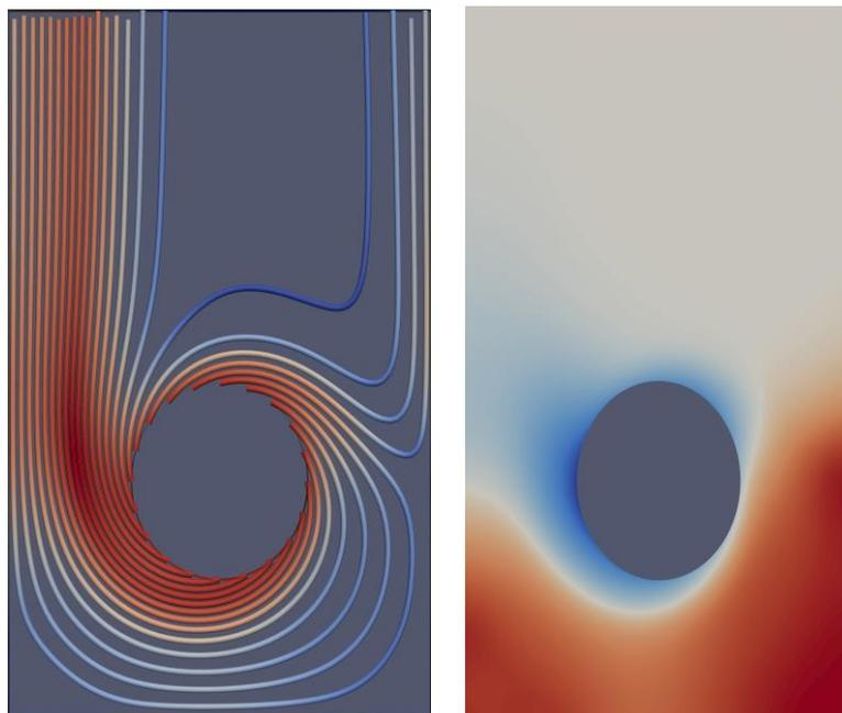
Figure 8: Flow patterns slow runner  $s/D = 1.2$ . Streamlines (left) coloured by velocity magnitude, pressure distribution (right). (Colour map: Maximum values red minimum values blue)
