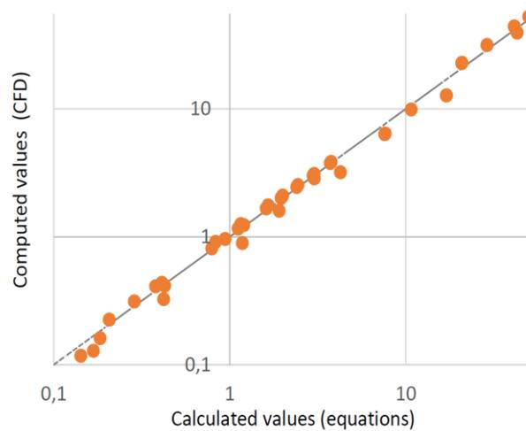
Figure 10: Correlation of computed and calculated values for the pressure difference as a function of enclosure size
