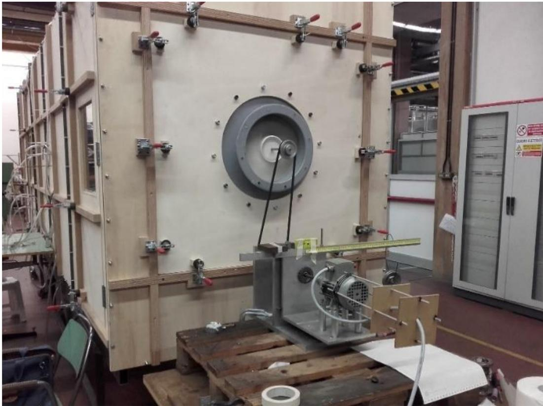
Figure 4: Inlet chamber test rig used for the tests. The picture was taken during the FSW test.
