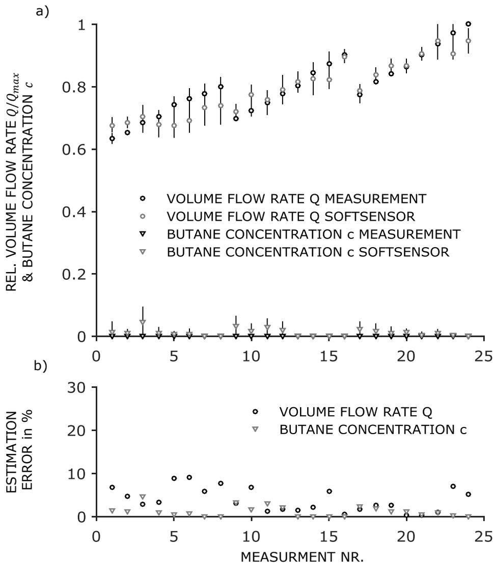
Figure 5: measured data and calculated values (a) and the resulting estimation errors (b)
