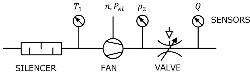
Figure 1: Test Rig Design
